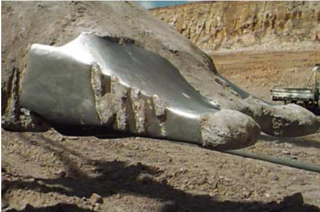
Appendix 14: A.R.M* Hardfaced quick tip after approximately 550 000 BCMs at BHP Gregory – still going fine.
