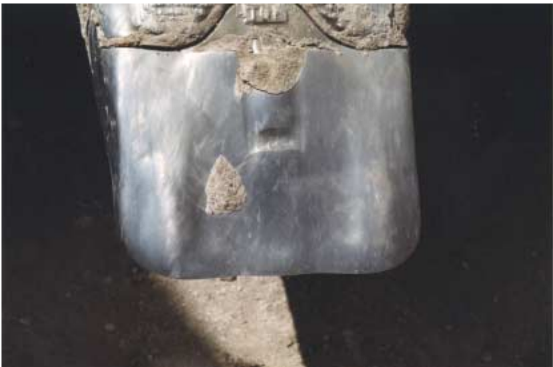
Appendix 13: Standard ESCO quicktip worn out after approx. 25,000 BCMs (not at BHP Gregory)
