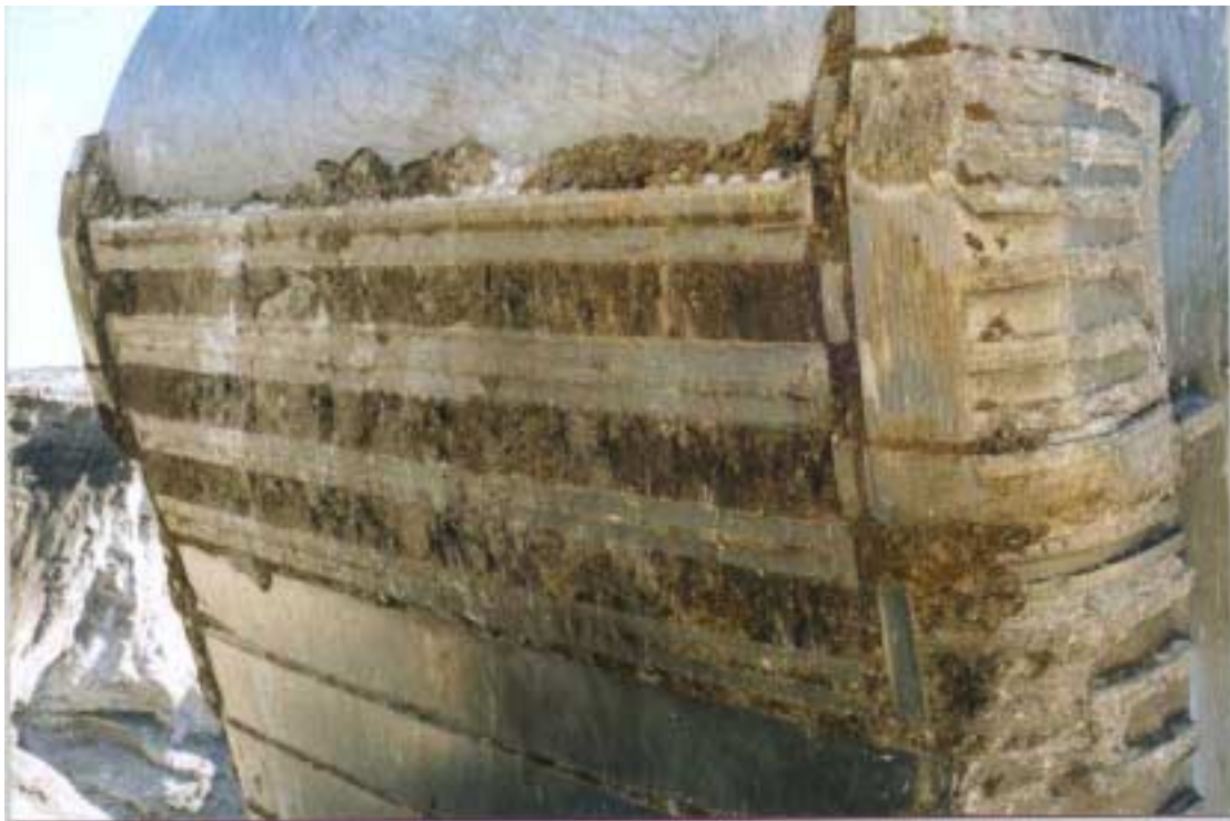
Figure 6.4 A.R.M.'s Heel Package on a P&H Bucket after 14 million BCMs
