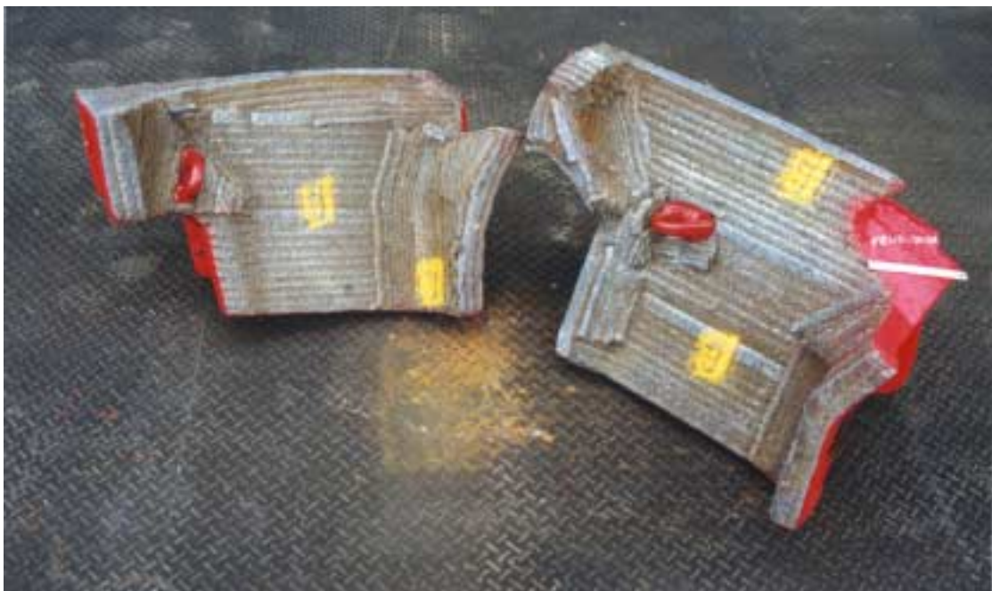
Appendix 7: A.R.M* Hardfaced wingshrouds
