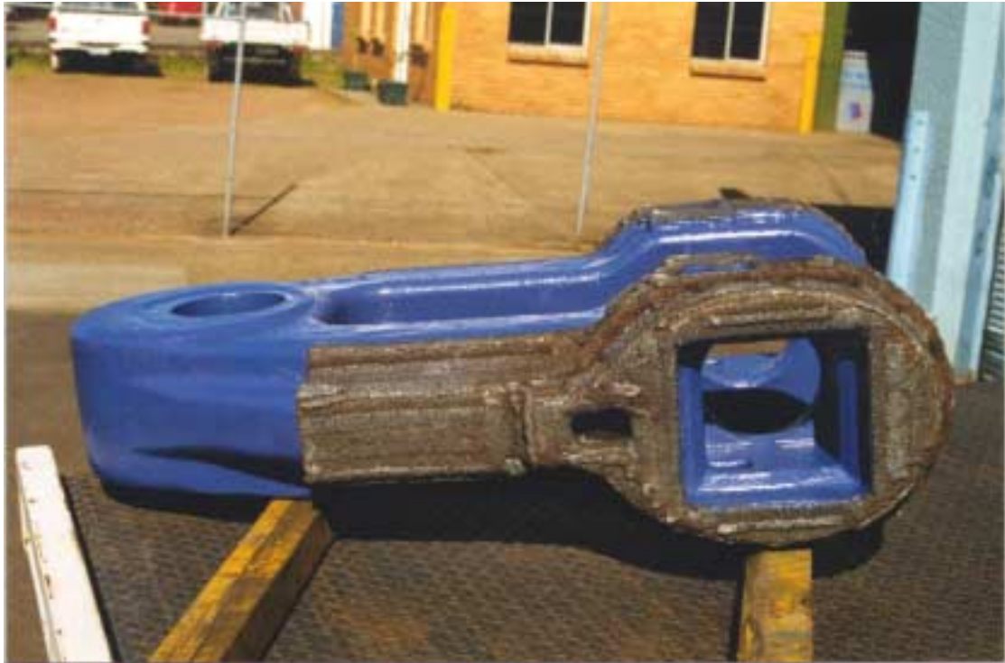
Appendix 10: A.R.M* hardfaced dragline shackle
