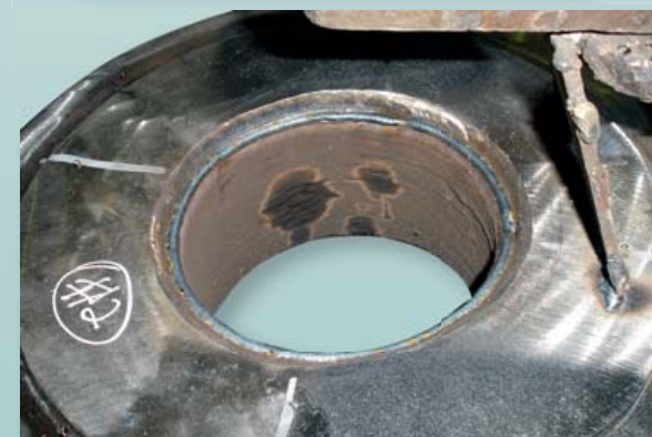
RS8750 – 06.1 – 8750 small bore rewelded – then machined for the bush install.
