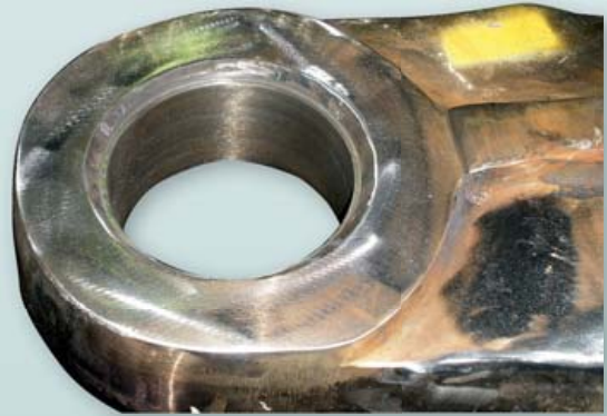
RS04 – 1350 small bush bore machined after a resize and welding.
