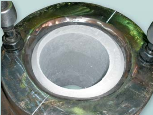
RS05 – 1350 Large Rope socket bush installed using Liquid Nitrogen.
