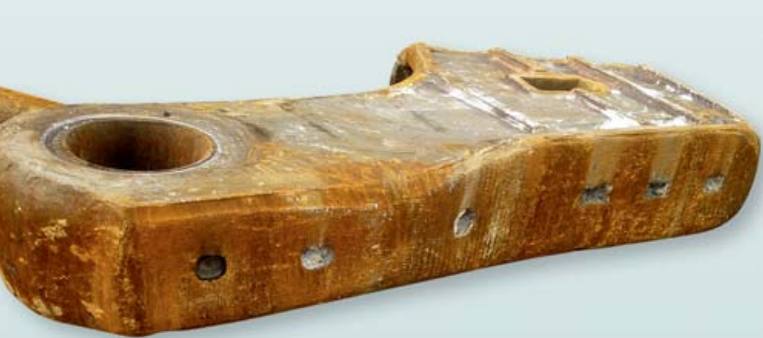
RS8750 – 02 – before the 3rd rebuild using A.R.M.* wear strips – has just completed 12 months of service.
