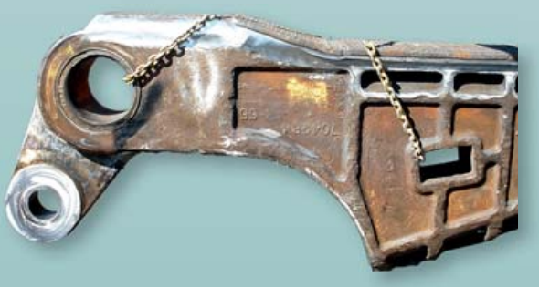
8750 rope socket totally rebuilt by A.R.M.*
