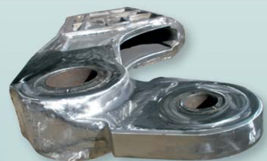
RS8750 – 05.3 – A.R.M.* Modification to strengthen the dump rope lug on the 8750 rope sockets.
