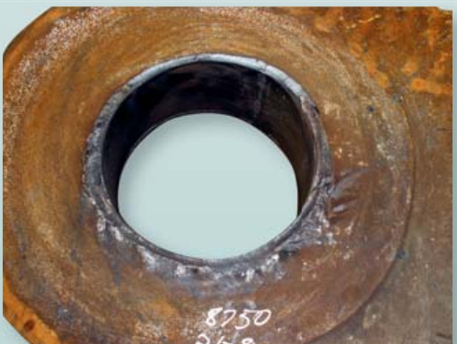
RS8750 – 05.2 – This photo shows the success of the A.R.M.* modification with no elongation of small bush bore after 12 months of service.
