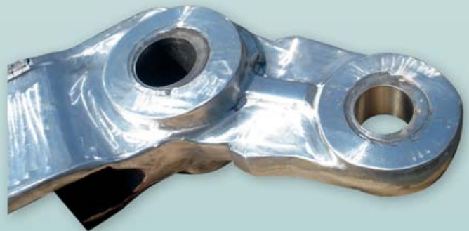
RS06 – 1350 rope socket Dump Lug upsized modification by A.R.M.*.
