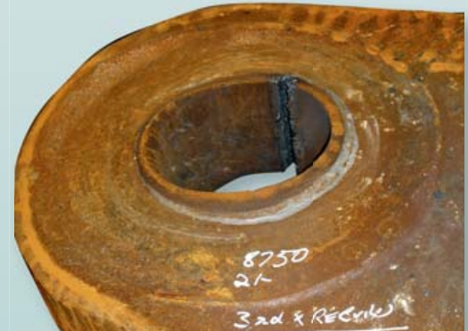
RS8750 – 05.1 – 8750 Small bush lug wear after modification by A.R.M.*
