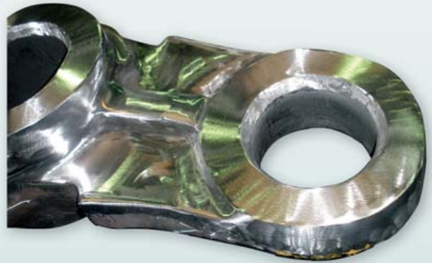
RS02 – 1350 Overview of the upsized modification on a 1350 small bush rebuild prior to line boring.
