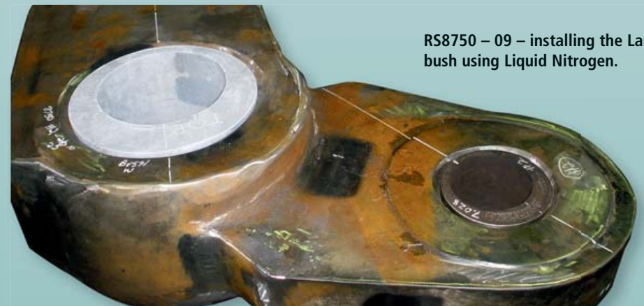
RS8750 – 07 – The Bush boss has been rebuilt back to as new.
