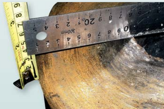
RS8750 – 05 – Worn 35mm per side on the Dump Rope Small Bush boss on each side.
