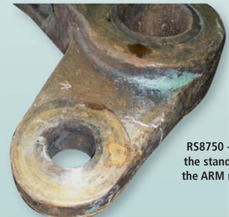
RS8750 – 05 – Worn 35mm per side on the Dump Rope Small Bush boss on each side.
