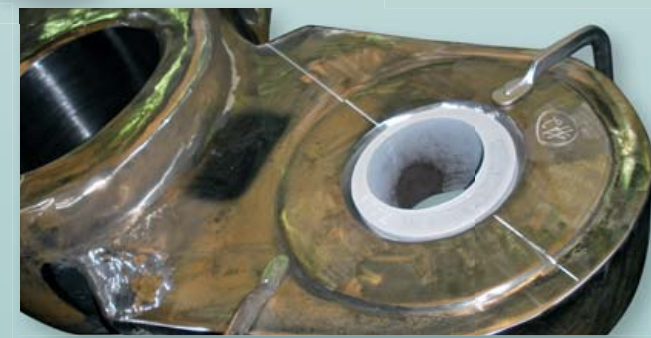
RS8750 – 07.1 – The rope socket AFTER modification to small bush lug.
