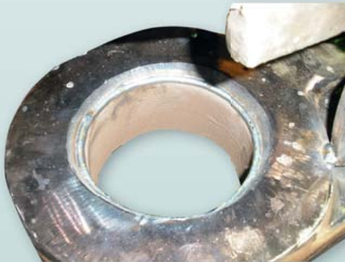
RS03 – 1350 small bush bore internally weld repaired.
