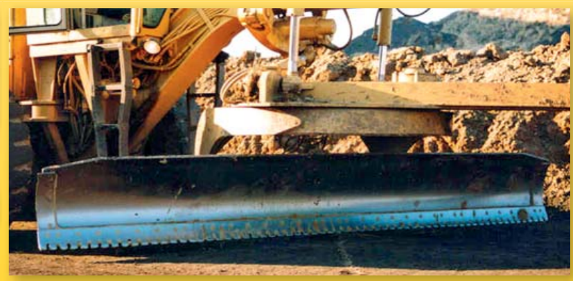
Overview of the new A.R.M.* Serrated Edge after 500 hours.
