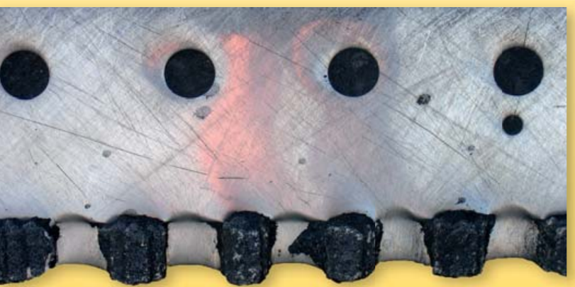
A.R.M.* 24M Semi-Serrated at 3,500 hours.
