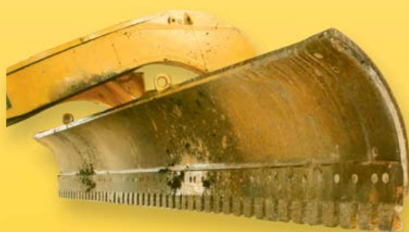
A.R.M.* 24H Serrated after 600 hours.
