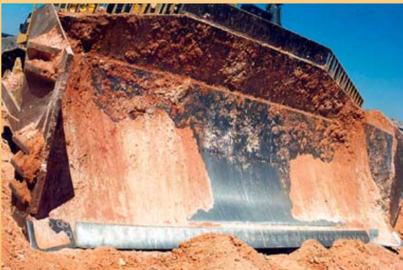
Standard 575 Blade – edges only last around 1,000 Hours.
