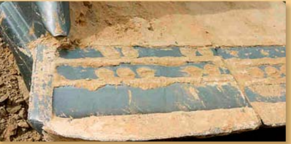
Patented A.R.M.* Carry Dozer edges after 5,020 hours.
