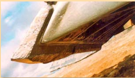
Patented A.R.M.* D11 Premium edges at 2,570 hours – not yet turned. Total life = 10,000 hours.
