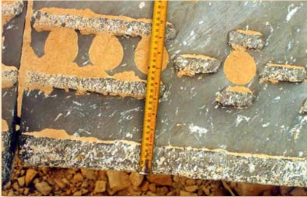
Patented A.R.M.* D11 Premium edges at 2,570 hours – not yet turned. Total life = 10,000 hours.
