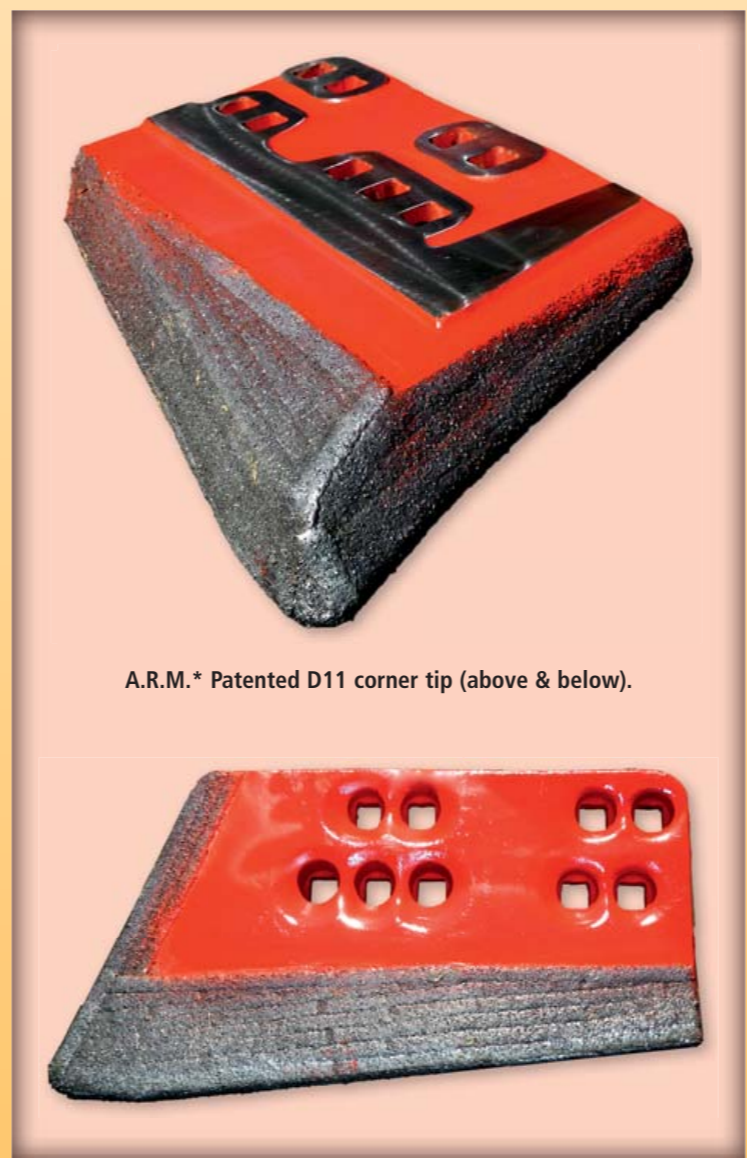
Patented A.R.M.* Carry Dozer edges after 5,020 hours.
