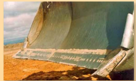
Left and Right: D11 – Patented A.R.M.* Premium Edges after 12,000 hours – not yet turned.
