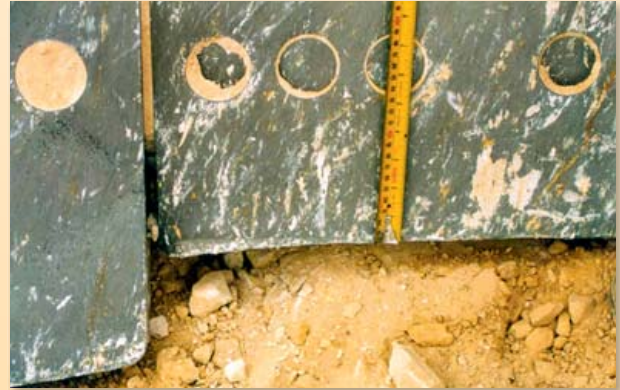
Cat A.R.M.* HF edges turned and worn out after a total life of 2,500 hours in the D11 trial.
